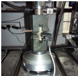
Figure.3. CTOD Testing Machine
