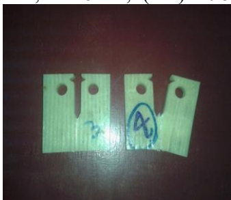
Figure.4. Specimen after CTOD test
