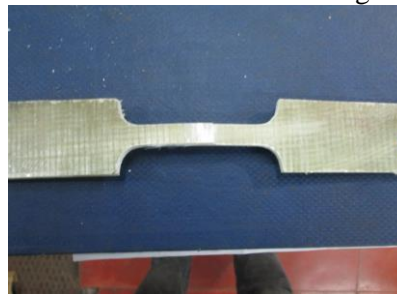
Figure.2. Specimen after tensile test
